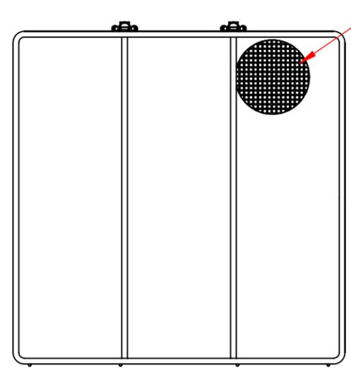
Lined Bottom, Sides, and Lid with 4 Mesh x .063" Woven Wire (.187" Openings, 56% Open Area)
